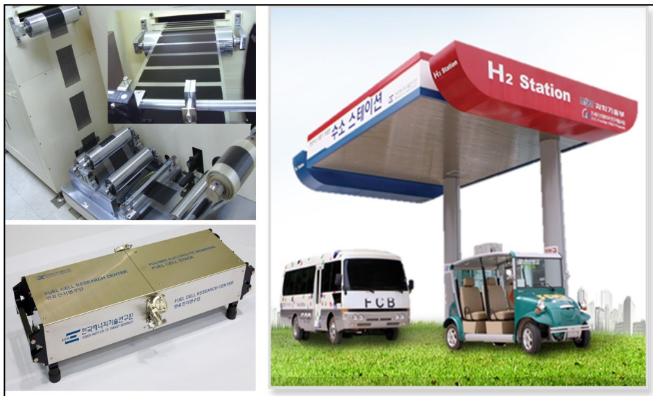
Roll to roll MEA fabrication process, 50 kW Stack for Fuel Cells mini-bus and Hydrogen refuelling station of KIER.
