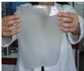
Scaled-up membrane at CNR-ITAE with a maximum dimension of 600 cm 2 .
