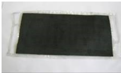
MEA with a maximum active area of 200 cm 2 .
