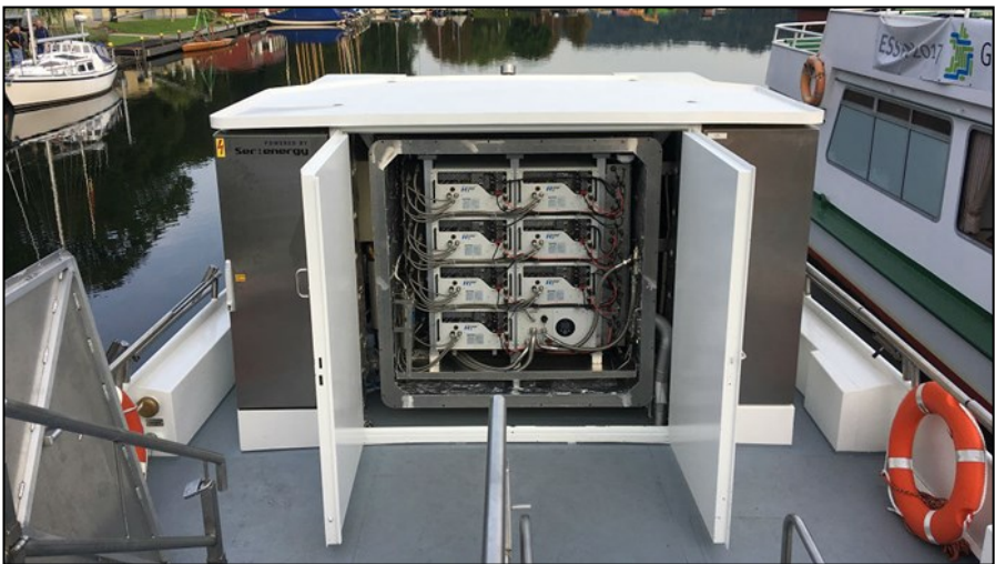
MS-Innogy is powered by seven 5 kW methanol fuel cells.
