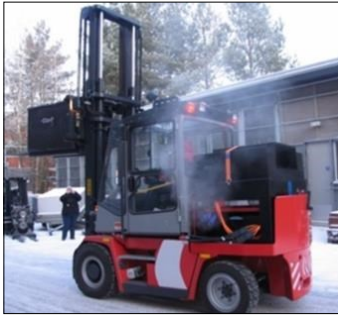
Electric forklift installed with PEMFC triple-hybrid power source.
