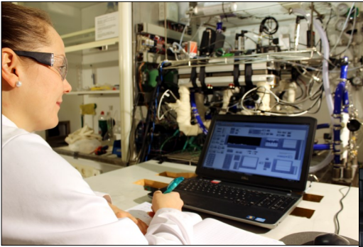
2 kW miniature automotive system, a unique hardware for contaminant studies in realistic conditions.
